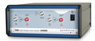
HIGH VOLTAGEFIXED GAINBROADBAND±200V20xDC to ca 500 kHz150mADC to ca 500 kHzFULL SCALELOW OUTPUT IMPEDANCEHIGH SLEW RATE<0.1 Ω</td>400 V/µs
