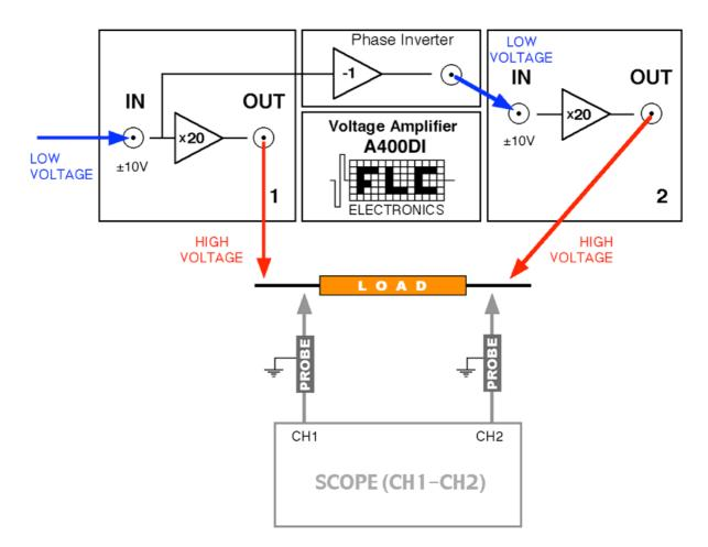
Observe, that both sides of the connected load are actively driven and must be isolated from the ground. The voltage over the load is in this case  $U_1 - U_2 = U_1 - (-U_1) = 2U_1$  since  $U_2 = -U_1$ .
