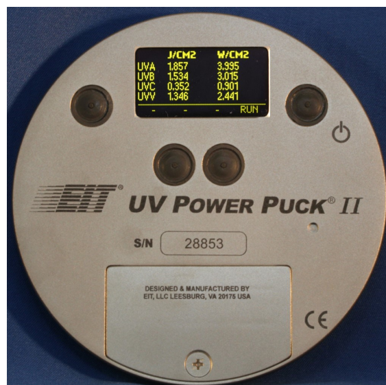
UV Power Puck II A four band radiometer
