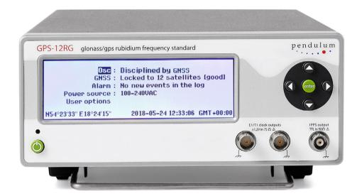
The Pendulum GPS-12RG Portable Reference clock is an ultra-stable GLONASS and GPS-disciplined Rubidium reference, targeted for both laboratory and telecommunications applications. The built-in battery option enables transportation of lab accuracy to field applications. When locked to GLONASS and/or GPS, its near-Cesium performance makes the GPS-12RG an ideal calibrator for metrology and test systems.
