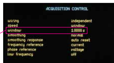
Example of setting the window, eg (50Hz set to 20ms)
