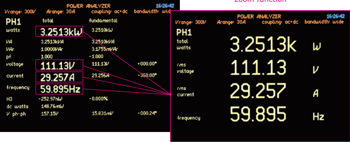
Zoom function enabled on total watts, rms voltage, rms current and frequency
