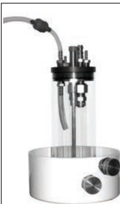
Figure 7: The RAD AQUA provides continuous fast-response measurement of radon and thoron in a water supply.
