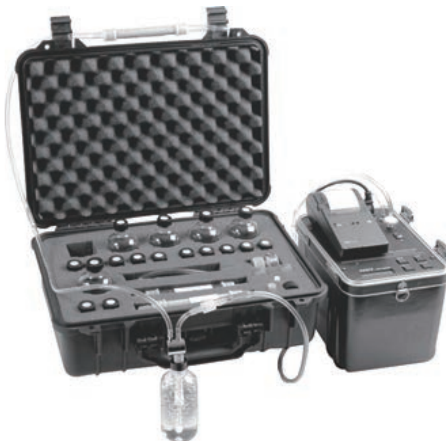
Figure 6: The RAD H 2 O accessory connected to a RAD7.
