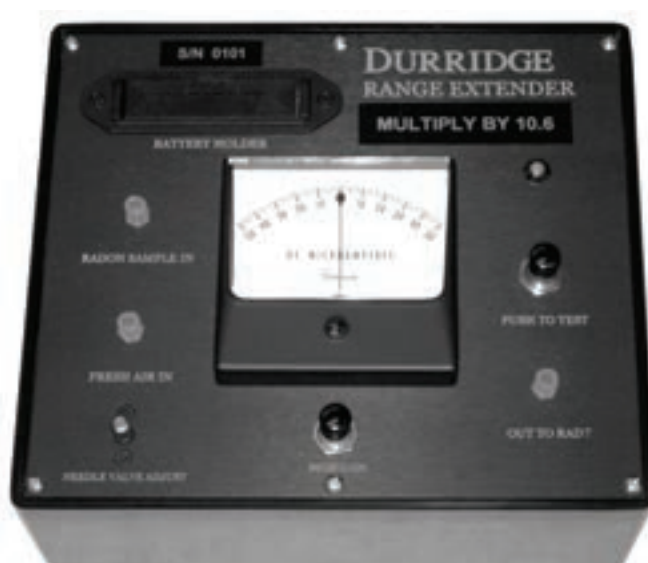
Figure 12: DURRIDGE Range Extender. The radon concentration delivered to the RAD7 is reduced by a factor of 10. The pump can cycle on and off without affecting the reduction factor.
