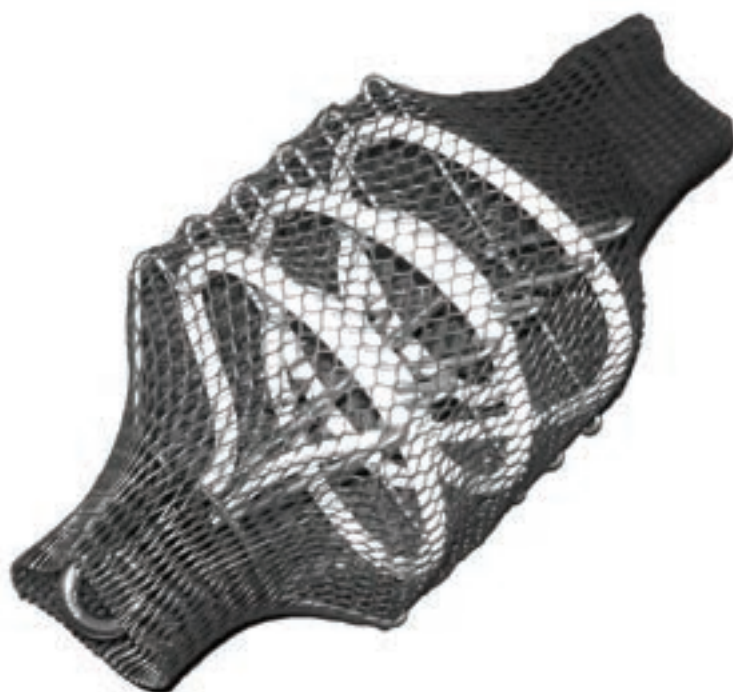
Figure 8: The Water Probe, for slow response monitoring of radon.
