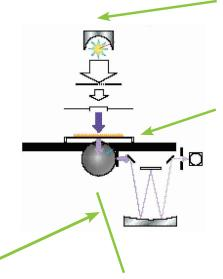
Ultraviolet (UVB) and near ultraviolet (UVA) radiation is provided by a 125W CW Xenon arc lamp.
