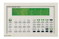
The UPC controller is a 3-Phase AC arbitrary waveform generator and precision AC metering system. Each waveform stored in the UPC is encoded with 12-bit amplitude and 10-bit time resolution for each cycle. The waveform for each phase may be independently selected and varied in amplitude and phase angle with respect
