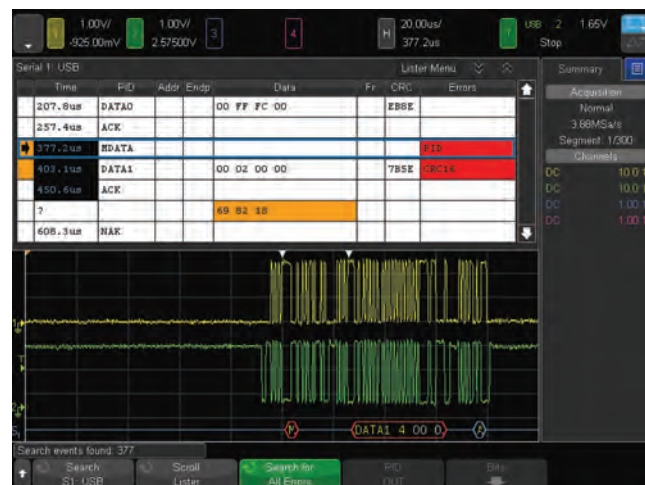
Figure 21. USB 2.0 trigger, decode and "lister" display.
