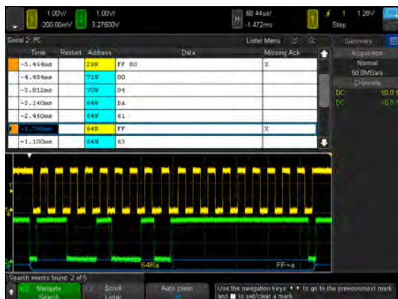
Figure 11. Using the error condition search, the 4000 X-Series quickly found 5 places with a missing acknowledgment in an I 2 C serial bus. The navigation feature moves between the errors and zooms automatically to show the error packet.
