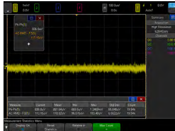
Figure 42. Getting 113 \mu\text{Vrms} noise floor at 1 mV/div with the high resolution mode.
