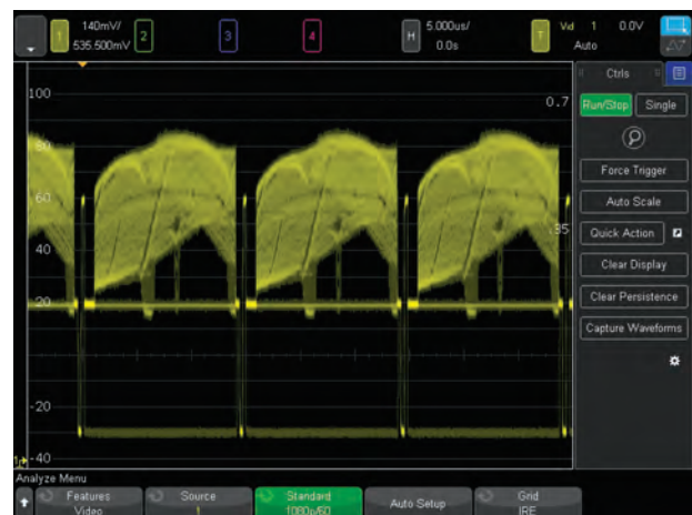
Figure 27. Triggering on 1080p HDTV signal analysis.
