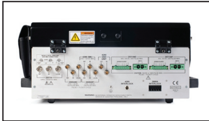
Flexible, safe test fixture for 3kV and 100A.
