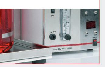
The FerMac 368 Gas Analyser measures oxygen and carbon dioxide in exit gas, two important extra parameters which give the best indication of growth within a fermenter vessel.
