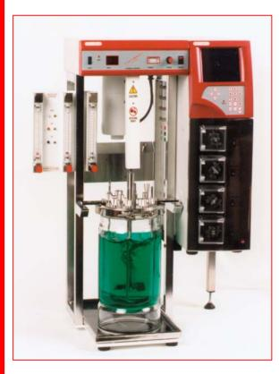
The stirrer is fitted with a reduction drive which provides constant low speeds and also protects the motor against wear and tear.
