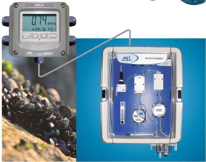
Potassium Permanganate (KMnO<sub>4</sub>) is a strong oxidizer used in the water industry for reduction of organics in raw water. It is also used for control of zebra mussel problems at raw water intake structures. Continuous monitoring of low permanganate concentrations allows operators to adjust chemical feed rates and achieve target values. Chemical feed problems that result in either too little or too much residual can be quickly identified and corrected.
