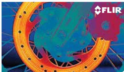
Motorcycle brake testing
