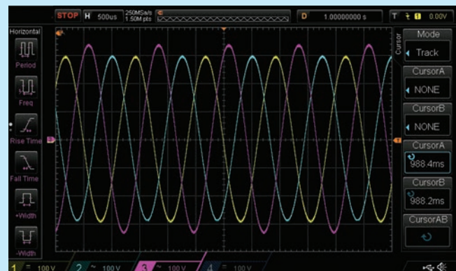
Three Phase Unbalance Voltage Test Captured
