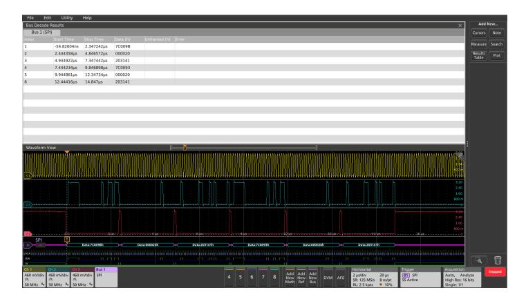
For firmware engineers, the Results Table format may be more usable. This time-stamped display of bus activity can be easily compared to software listings, and allows easy calculation of the execution speed.
