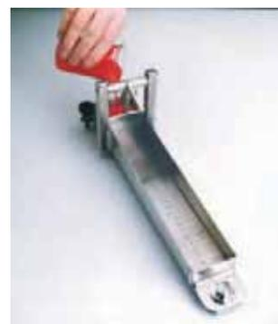
The gate is released, by pressing the lock release lever, while the spring action ensures it opens instantaneously.
