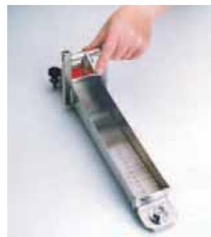
As the fluid flows down the instrument its progress can be accurately measured using the graduated scale. By comparing the flow rate to specified time periods the physical properties of the sample can be calculated.
