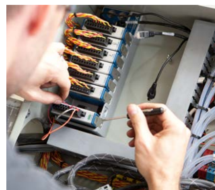
CompactDAQ in an industrial enclosure as part of engine test cell
