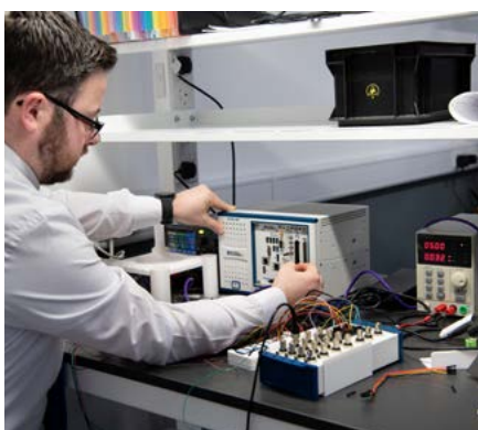
PXI used for benchtop validation system
