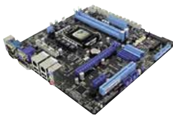
▲ MICRO-ATX (244 x 244 mm)
