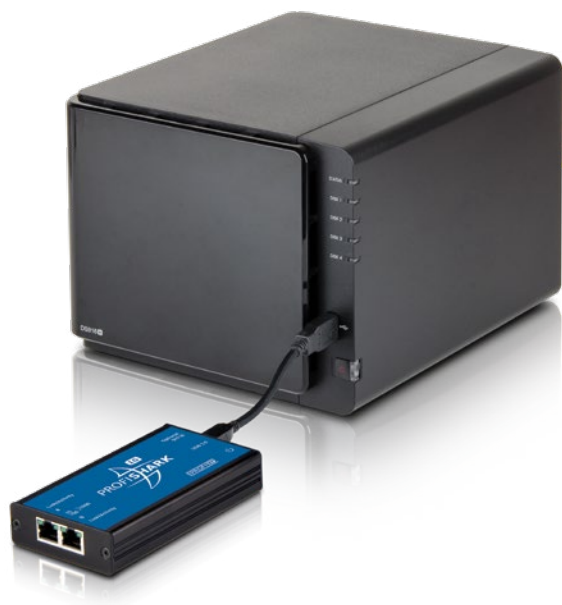
PROFISHARK LONG-TERM TRAFFIC CAPTURE SETUP
