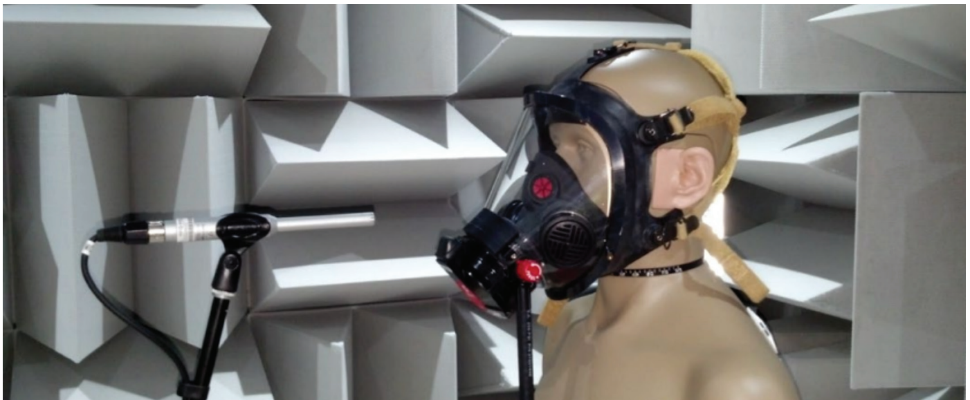
NFPA 1981 testing of self-contained breathing apparatus, SCBA, mounted on a G.R.A.S. KEMAR manikin in an anechoic chamber. [Photo courtesy of Scott Safety, used by permission; for illustration only, not to scale.]
