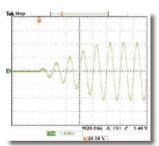
The Rise time control function enables you to increases the test voltage gradually to reach the setting voltage while the AC Hipot (Withstanding voltage) test is conducted. The voltage rise time can be set from 0.1s to 10.0s at a resolution of 0.1s.
