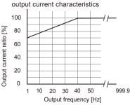
For the "Output voltage ratio versus rated output current characteristics (AC mode)" and "Load power factor versus rated output current characteristics" graphs, the rated output current is the product of the output current ratios shown in both graphs. The output current ratio shown in the "Output frequency versus rated output current characteristics" graph is given priority if it is less than the product of the output current ratios described above. (This only applies to AC mode.)
