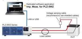
Measurement condition diagram
