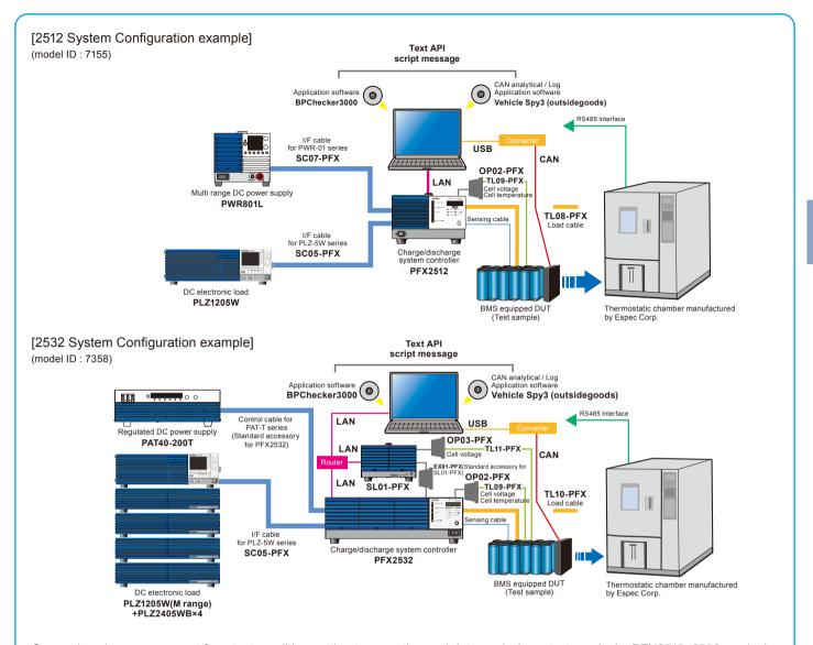
Comprehensive management from test condition setting to execution and data analysis on test results by PFX2512, 2532 exclusive application software, BPChecker3000
