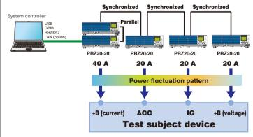
Example of combined trigger- and clocksynchronized operation
