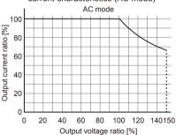
■ Output voltage ratio versus rated output
