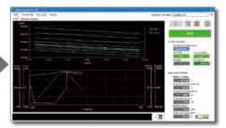
When the operation starts, the interpolated I-V file that will be simulated is selected, and control operating points are plotted in orange.
