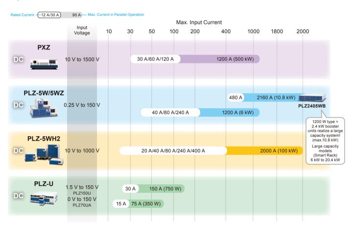
High-Capacity Regenerative Electronic Load (CC/CV/CR/CP)
