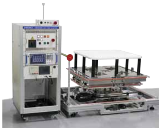
Automatic position control of power transmission coil (max. 800 mm)
