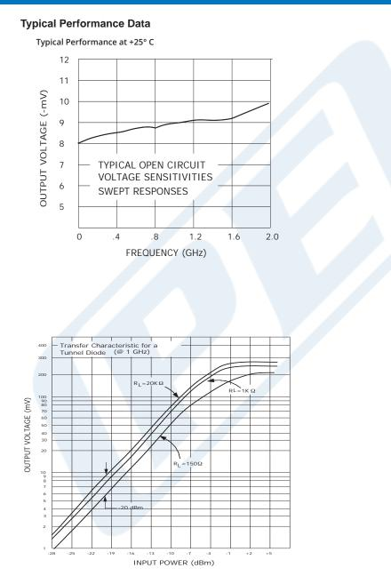
Click the following link (or enter part number in "SEARCH" on website) to obtain additional part information including price, inventory and certifications: Tunnel Diode Detector, SMA, 5 nsec Pulse Risetime, Positive Video Out, +17 dBm max Pin, 100 MHz to 2 GHz PE80T6001
