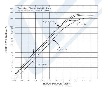
Click the following link (or enter part number in "SEARCH" on website) to obtain additional part information including price, inventory and certifications: Tunnel Diode Detector, SMA, 5 nsec Pulse Risetime, Negative Video Out, +17 dBm max Pin, 100 MHz to 4 GHz PE80T6002
