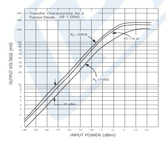
Click the following link (or enter part number in "SEARCH" on website) to obtain additional part information including price, inventory and certifications: Tunnel Diode Detector, SMA, 5 nsec Pulse Risetime, Negative Video Out, +17 dBm max Pin, 500 MHz to 18 GHz PE80T6004
