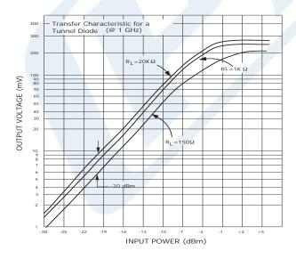
Click the following link (or enter part number in "SEARCH" on website) to obtain additional part information including price, inventory and certifications: Tunnel Diode Detector, SMA, 5 nsec Pulse Risetime, Positive Video Out, +17 dBm max Pin, 500 MHz to 18 GHz PE80T6005
