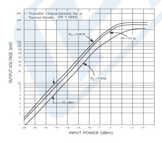
Click the following link (or enter part number in "SEARCH" on website) to obtain additional part information including price, inventory and certifications: Tunnel Diode Detector, SMA, 5 nsec Pulse Risetime, Negative Video Out, +17 dBm max Pin, 2 GHz to 18 GHz PE80T6006
