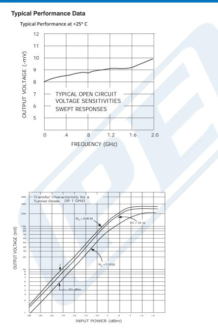
Click the following link (or enter part number in "SEARCH" on website) to obtain additional part information including price, inventory and certifications: Tunnel Diode Detector, SMA, 5 nsec Pulse Risetime, Positive Video Out, +17 dBm max Pin, 2 GHz to 18 GHz PE80T6007
