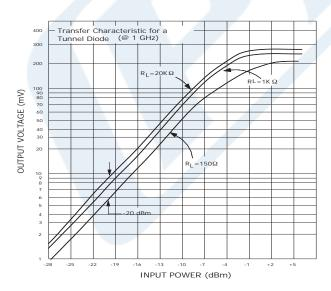
Click the following link (or enter part number in "SEARCH" on website) to obtain additional part information including price, inventory and certifications: Tunnel Diode Detector, SMA, 5 nsec Pulse Risetime, Negative Video Out, +17 dBm max Pin, 2 GHz to 6 GHz PE80T6016
