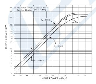
Click the following link (or enter part number in "SEARCH" on website) to obtain additional part information including price, inventory and certifications: Tunnel Diode Detector, SMA, 5 nsec Pulse Risetime, Negative Video Out, +17 dBm max Pin, 6 GHz to 12 GHz PE80T6020
