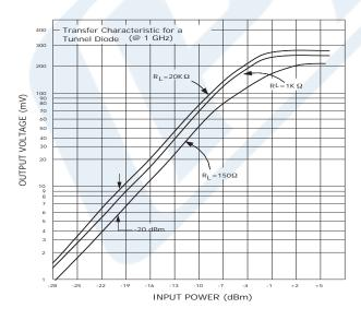
Click the following link (or enter part number in "SEARCH" on website) to obtain additional part information including price, inventory and certifications: Tunnel Diode Detector, SMA, 5 nsec Pulse Risetime, Negative Video Out, +17 dBm max Pin, 18 GHz to 26 GHz PE80T6024
