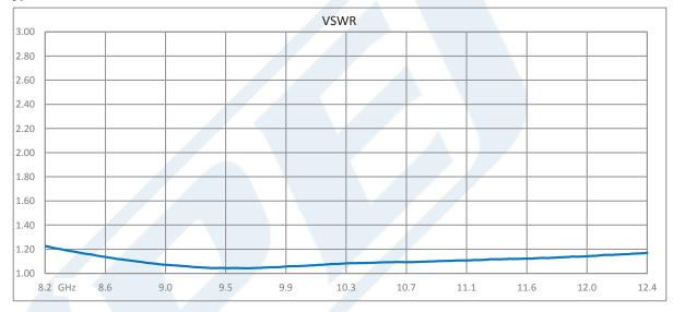
WR-90 CPR-90G Grooved Flange to N Female Waveguide to Coax Adapter Operating from 8.2 GHz to 12.4 GHz from Pasternack Enterprises has same day shipment for domestic and International orders. Our RF, microwave and millimeter wave products maintain a 99.4% availability and are part of the broadest selection in the industry.
