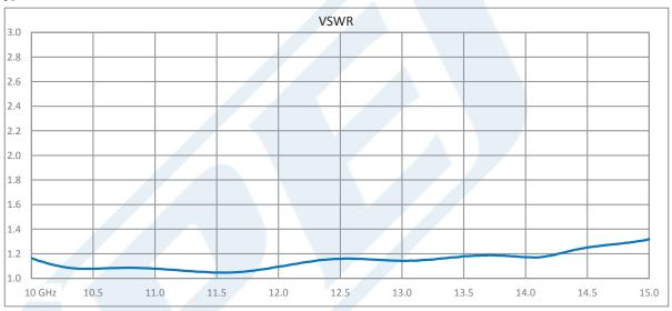
WR-75 Square Cover Flange to End Launch SMA Female Waveguide to Coax Adapter, 10 GHz to 15 GHz, M Band, Aluminum, Paint from Pasternack Enterprises has same day shipment for domestic and International orders. Our RF, microwave and millimeter wave products maintain a 99.4% availability and are part of the broadest selection in the industry.
