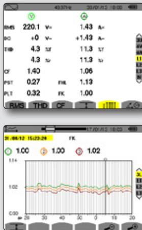
The harmonic currents flowing in a network lead to increased losses in the windings. This results in heating of the transformer and reduces the life span of the instruments connected.
