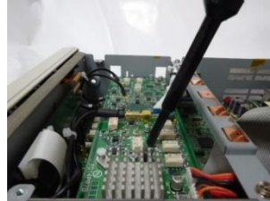
The measurement of conventional electric field probe
