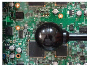
General sphere electric probe, diameter: 3cm
