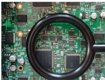
General loop magnetic probe , diameter: 6.8cm
