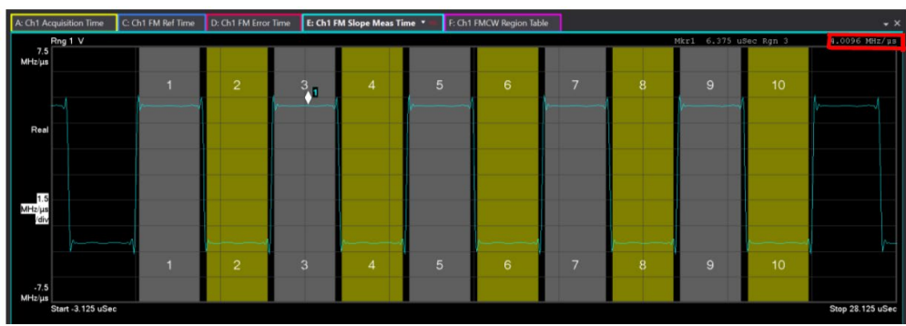
The FM slope time analysis in figure 8 measures the steepness of the modulation. Ideally, the slope is a perfect square wave. The slope is ~4MHz/us. It can be calculated with below formula.
