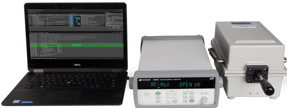
Figure 13. X8711A IoT device functional test solution
