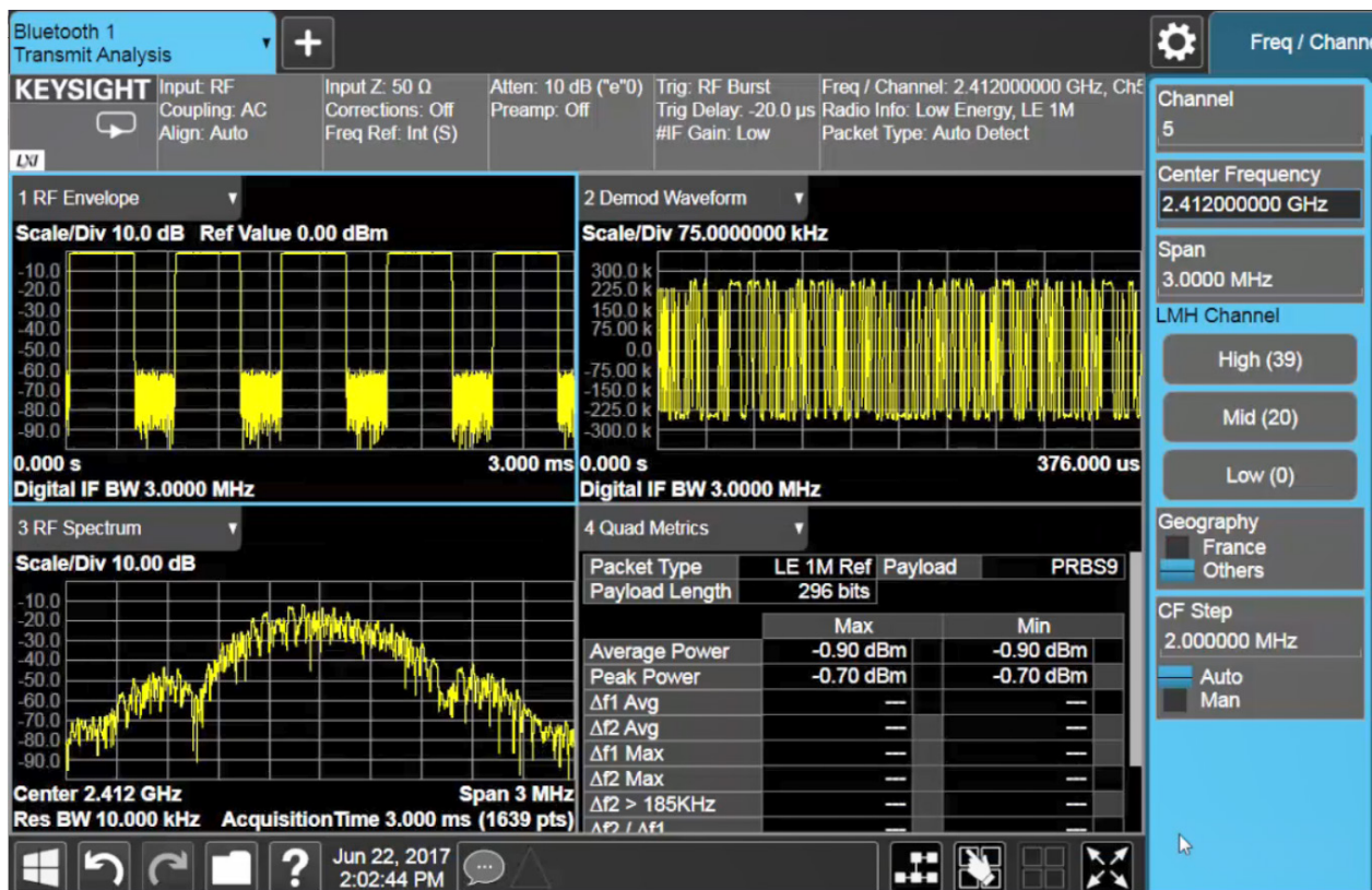
Figure 7. Quad-view display of Bluetooth® 5 PHY (LE 1M) using N9081C Bluetooth® measurement application running in the Keysight N9000B CXA Signal Analyzer
