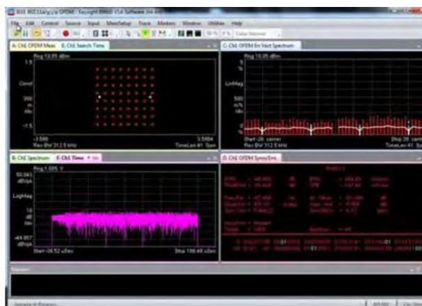
Using data acquired from S-Series, VSA shows an EVM for IEEE 802.11 QAM 64 of 0.47%.
