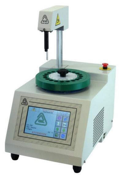
CryoTouch 20 is a 20-sample carousel-based automatic equipment for the rapid determination of the milk cryoscopic point variation caused by added water, in full compliance with the IDF-ISO 5764:2009 international reference standard.
