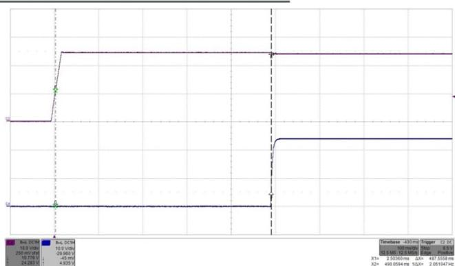
Fig. 34: Turn-on by  $V_{in}$  transient (ON/OFF high) at full rated load current (resistive) at  $V_{in} = 24V$ . Top trace (C2): Input voltage  $V_{in}$  (10 V/div.). Bottom trace (C4): Output voltage (10 V/div.). Time: 100 ms/div.
