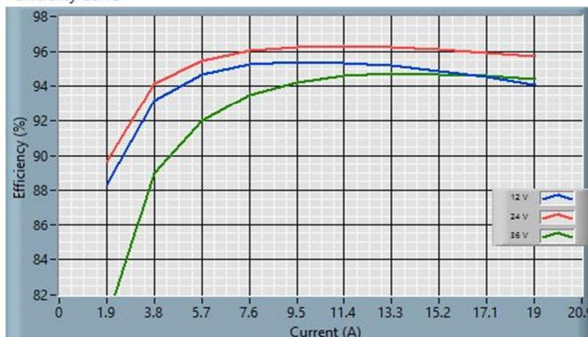
Fig. 15: 24S53.19FXW (ROHS) Efficiency Curve
