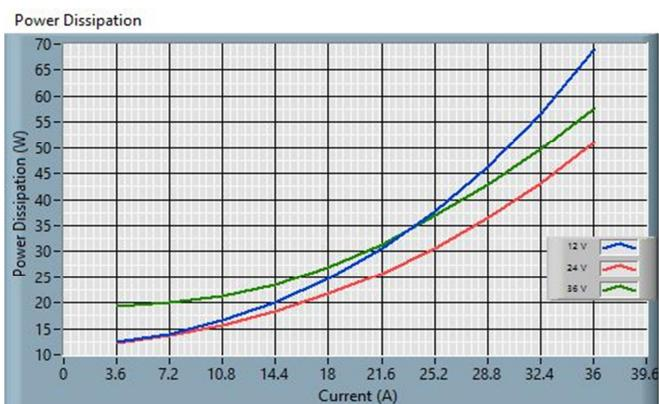
Fig. 12: 24S28.36FXW (ROHS) Power Dissipation
