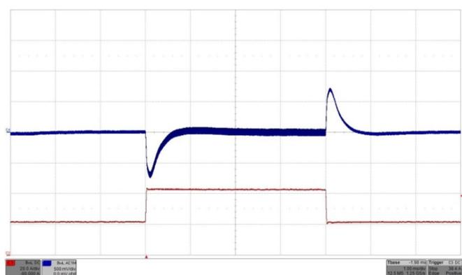
Fig. 36: Output voltage response to load current step change 50% - 100%- 50% (21A-42A-21A) with  $di/dt = 1A/\mu s$  at  $V_{in} = 24 V$ . Top trace (C4): Output voltage (500 mV/div.). Bottom trace (C3): Load current (20A/div.).  $C_o = 2 \times 470 \mu F/70m\Omega$ . Time: 1ms/div.
