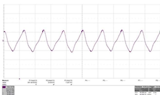
Fig. 50: Input reflected ripple current,  $i_c$  (500 mA/div.), measured at input terminals at full rated load current at Vin = 24 V. Refer to Fig. 2 for test setup. Time: 2  $\mu$ s/div. RMS input ripple current is  $7.3 \times 0.5A = 3.65A_{rms}$ .
