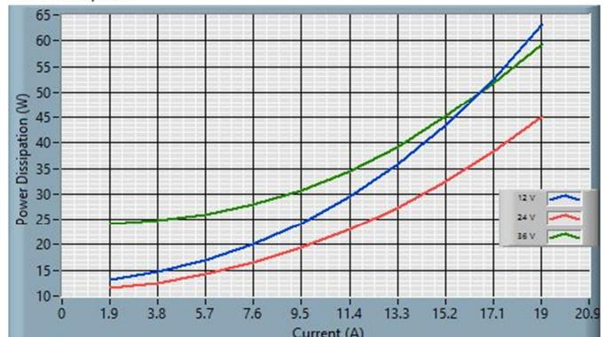
Fig. 16: 24S53.19FXW (ROHS) Power Dissipation
