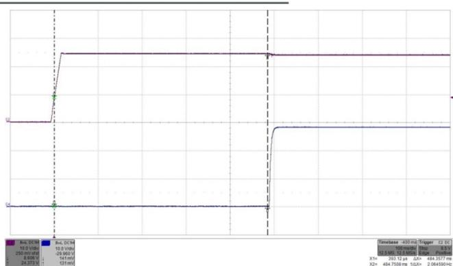
Fig. 40: Turn-on by Vin (ON/OFF high) transient at full rated load current (resistive) at Vin = 24V. Top trace (C2): Input voltage Vin (10 V/div.). Bottom trace (C4): Output voltage (10 V/div.). Time: 100 ms/div.
