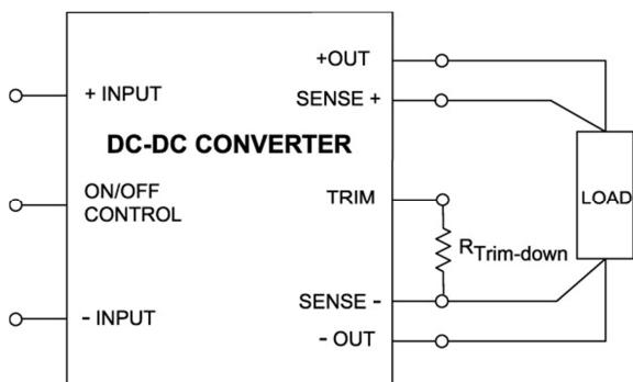
Fig. 3: Circuit configuration for Trim-down function
