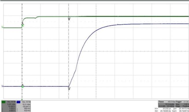
Fig. 51: Turn-on by ON/OFF transient (Vin applied) at full rated load current (resistive) at Vin = 24V. Top trace (C1): ON/OFF signal (5 V/div.). Bottom trace (C4): Output voltage (10 V/div.). Time: 10 ms/div.
