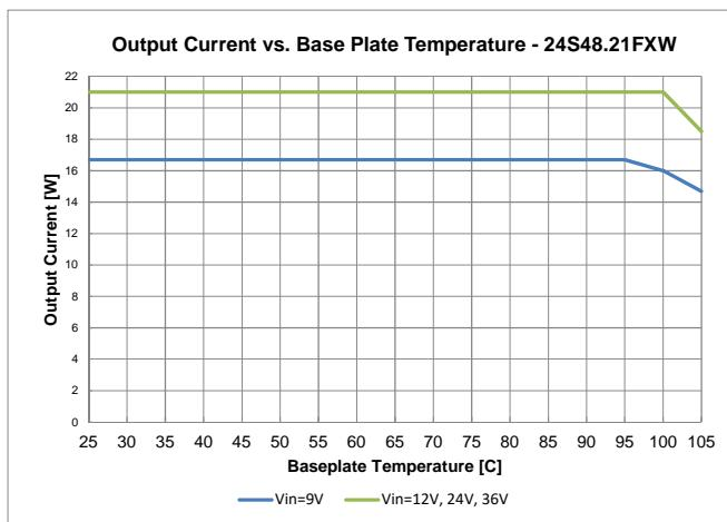
Fig. 24: 24S48.21FXW (ROHS) Derating Curve
