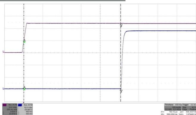
Fig. 46: Turn-on by Vin (ON/OFF high) transient at full rated load current (resistive) at Vin = 24V. Top trace (C2): Input voltage Vin (10 V/div.). Bottom trace (C4): Output voltage (10 V/div.). Time: 100 ms/div.
