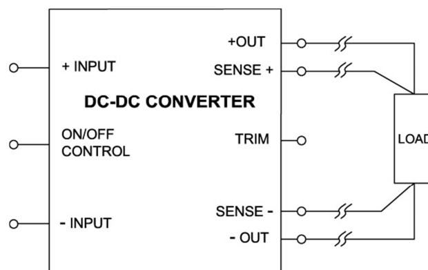
Fig. 2: Circuit configuration for Remote sense function.
