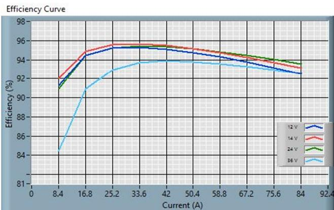
Fig. 7: 24S12.84FXW (ROHS) Efficiency Curve
