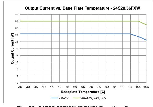
Fig. 22: 24S28.36FXW (ROHS) Derating Curve
