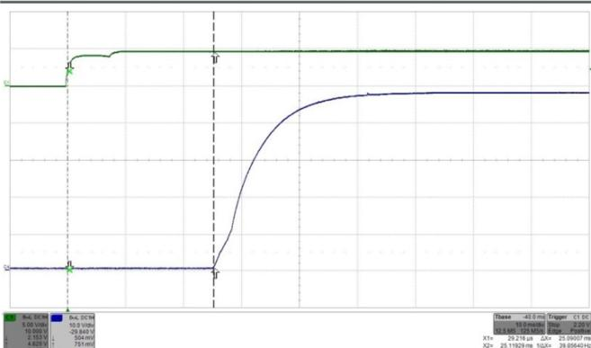
Fig. 45: Turn-on by ON/OFF transient (Vin applied) at full rated load current (resistive) at Vin = 24V. Top trace (C1): ON/OFF signal (5 V/div.). Bottom trace (C4): Output voltage (10 V/div.). Time: 10 ms/div..
