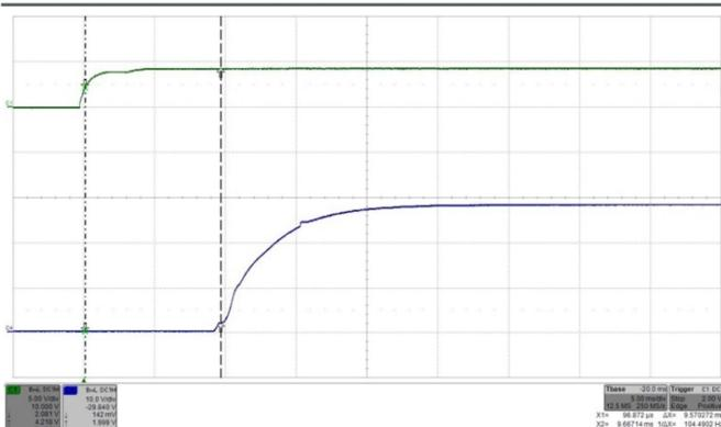
Fig. 39: Turn-on by ON/OFF transient (Vin applied) at full rated load current (resistive) at Vin = 24V. Top trace (C1): ON/OFF signal (5 V/div.). Bottom trace (C4): Output voltage (10 V/div.). Time: 5 ms/div.
