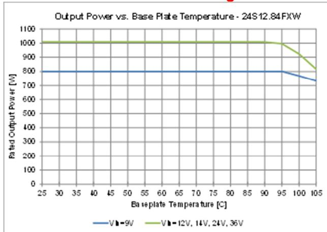
Fig. 17: 24S12.84FXW (ROHS) Derating Curve
