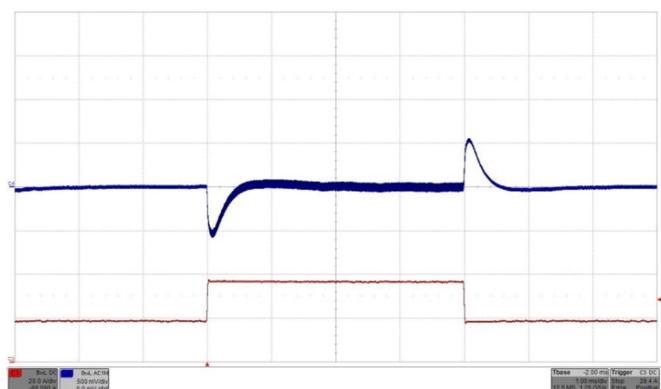
Fig. 42: Output voltage response to load current step change 50% - 100%- 50% (18A-36A-18A) with  $di/dt = 1A/\mu s$  at Vin = 24V . Top trace (C4): Output voltage (500 mV/div.). Bottom trace (C3): Load current (10A/div.).  $C_o = 470\mu F/70m\Omega$ . Time: 1ms/div.
