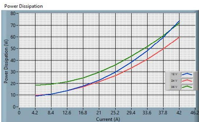
Fig. 10: 24S24.42FXW (ROHS) Power Dissipation
