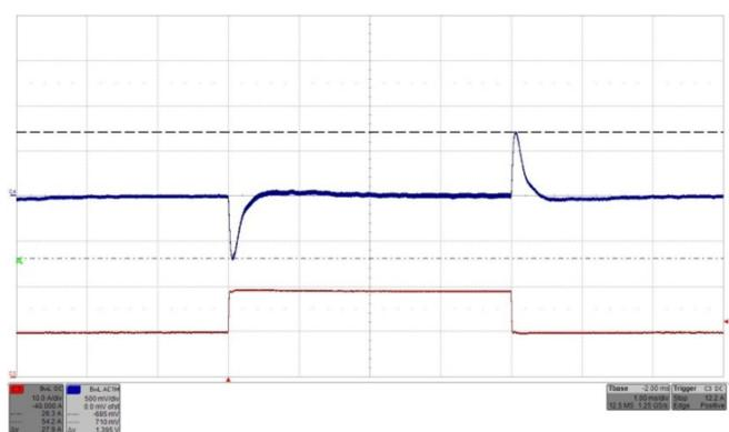
Fig. 54: Output voltage response to load current step change 50% - 100%- 50% (9.5A-19.25A-9.5A) with  $di/dt = 1A/\mu s$  at Vin = 24V . Top trace (C4): Output voltage (500 mV/div.). Bottom trace (C3): Load current (10A/div.). Time: 1ms/div.
