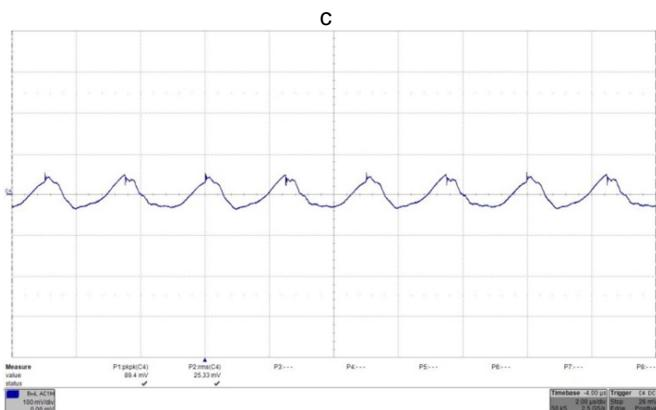
Fig. 43: Output voltage ripple (100 mV/div.) at full rated load current into a resistive load at Vin = 24 V.  $C_o = 470\mu F/70m\Omega$ . Time: 2  $\mu s$ /div.
