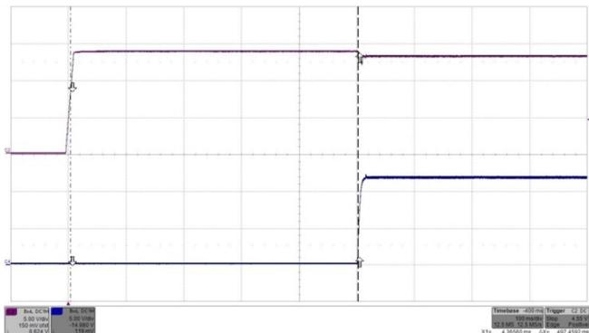
Fig. 28: Turn-on by  $V_{in}$  transient (ON/OFF high) at full rated load current (resistive) at  $V_{in} = 44V$ . Top trace (C2): Input voltage  $V_{in}$  (5 V/div.). Bottom trace (C4): Output voltage (5 V/div.). Time: 100 ms/div.
