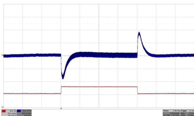
Fig. 35: Output voltage response to load current step change 50% - 75%- 50% (21A-31.5A-21A) with  $di/dt = 1A/\mu s$  at  $V_{in} = 24V$ . Top trace (C4): Output voltage (200 mV/div.). Bottom trace (C3): Load current (20A/div.).  $C_o = 470\mu F/70m\Omega$ . Time: 1ms/div.
