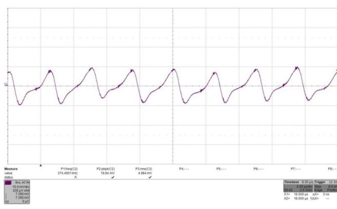
Fig. 56: Input reflected ripple current,  $i_c$  (500 mA/div.), measured at input terminals at full rated load current at Vin = 24 V. Refer to Fig. 2 for test setup. Time: 2  $\mu$ s/div. RMS input ripple current is  $4.968 \times 0.5A = 2.48A_{rms}$ .
