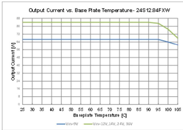
Fig. 18: 24S12.84FXW (ROHS) Derating Curve
