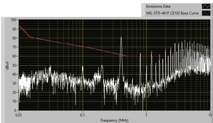
a) Without input filter from Fig. 47 (C9 = 2 x 470µF/50V/70mΩ)
