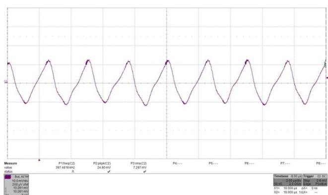
Fig. 38: Input reflected ripple current,  $i_c$  (500mA/mV), measured at input terminals at full rated load current at  $V_{in} = 24 V$ . Refer to Fig. 2 for test setup. Time: 2  $\mu s$ /div. RMS input ripple current is  $7.3 \times 0.5 A = 3.65 A_{rms}$ .
