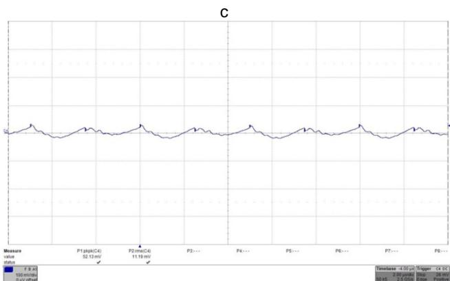
Fig. 55: Output voltage ripple (100 mV/div.) at full rated load current into a resistive load at Vin = 24 V. Time: 2  $\mu$ s/div.
