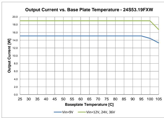
Fig. 26: 24S53.19FXW (ROHS) Derating Curve
