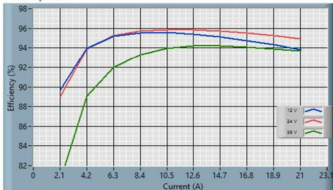
Fig. 13: 24S48.21FXW (ROHS) Efficiency Curve
