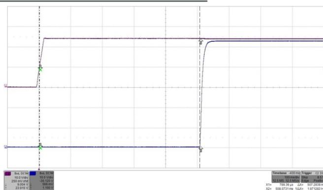
Fig. 52: Turn-on by Vin (ON/OFF high) transient at full rated load current (resistive) at Vin = 24V. Top trace (C2): Input voltage Vin (10 V/div.). Bottom trace (C4): Output voltage (10 V/div.). Time: 100 ms/div.
