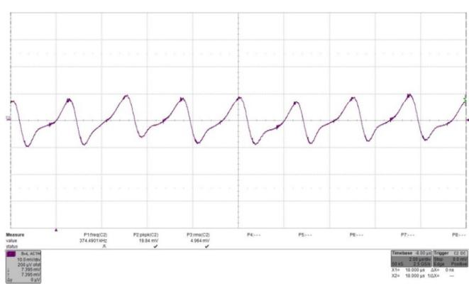
Fig. 44: Input reflected ripple current,  $i_C$  (500 mA/div.), measured at input terminals at full rated load current at Vin = 24 V. Refer to Fig. 2 for test setup. Time: 2  $\mu s$ /div. RMS input ripple current is  $4.968 \times 0.5A = 2.48A_{rms}$ .
