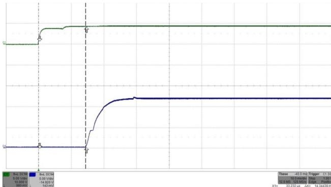
Fig. 27: Turn-on by ON/OFF transient (with  $V_{in}$  applied) at full rated load current (resistive) at  $V_{in} = 14V$ . Top trace (C1): ON/OFF signal (5 V/div.). Bottom trace (C4): Output voltage (5 V/div.). Time: 10 ms/div.
