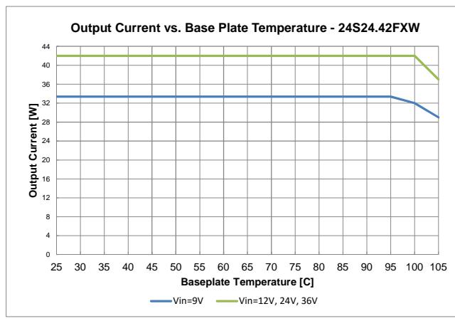
Fig. 20: 24S24.42FXW (ROHS) Derating Curve
