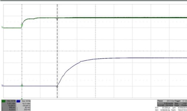
Fig. 33: Turn-on by ON/OFF transient (with  $V_{in}$  applied) at full rated load current (resistive) at  $V_{in} = 24V$ . Top trace (C1): ON/OFF signal (5 V/div.). Bottom trace (C4): Output voltage (10 V/div.). Time: 5 ms/div.
