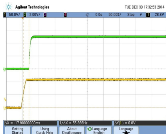
Turn-on transient at full load current (50 mS/div, Top Trace: Vout, 2V/div; Bottom Trace: Vin, 50V/div)
