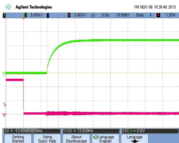
Figure 15: Turn-on transient at zero load current (10 mS/div, Top Trace: Vout, 5V/div; Bottom Trace: ON/OFF, 2V/div)
