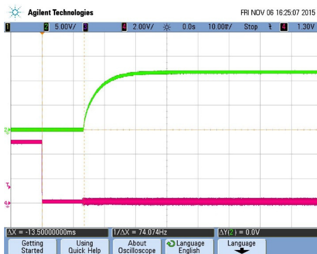
Figure 16: Turn-on transient at full load current (10 mS/div, Top Trace: Vout, 5V/div; Bottom Trace: ON/OFF, 2V/div)
