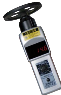
DT-207LR-S12 Contact Tachometer with Optional 12" Circle Wheel
