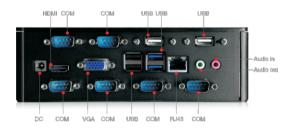
This system is equipped with display interfaces as HDMI(2048x1536/75HZ), VGA, allowing for multiple display and high definition effect.
