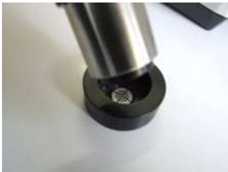
Target device for measurement area: 1.5, 4 or 6mm
