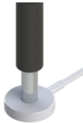
Figure 6. BlueWave® LED Prime using a 8-mm lightguide, measured directly on the surface of the radiometer
