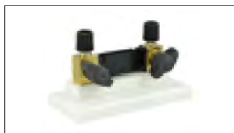
207030500: 0.001 ohm shunt, 0.5%, 50A max
