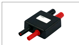
989007000: 50 ohms shunt, 0.1%, 0.05A max
