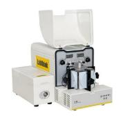
regulate and control the temperature, humidity and flow rate properly, which guarantee the testing sensitivity and repeatability of test results. C230 is applicable to determination of oxygen permeability of plastic films, sheeting, paper, packages and other relative packaging materials in food, pharmaceutical, medical apparatus, daily chemical, photovoltaic and electronic industries, etc.
