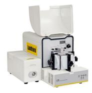
can regulate and control the temperature, humidity and flow rate properly, which guarantee the testing sensitivity and repeatability of test results. C330 is applicable to determination of water vapor permeability of plastic films, sheeting, paper, packages and other relative packaging materials in food, pharmaceutical, medical apparatus, daily chemical, photovoltaic and electronic industries, etc.
