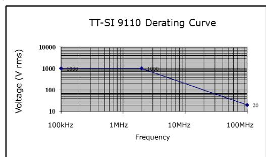
The derating curve of the absolute maximum input voltage in common mode is shown as follows.
